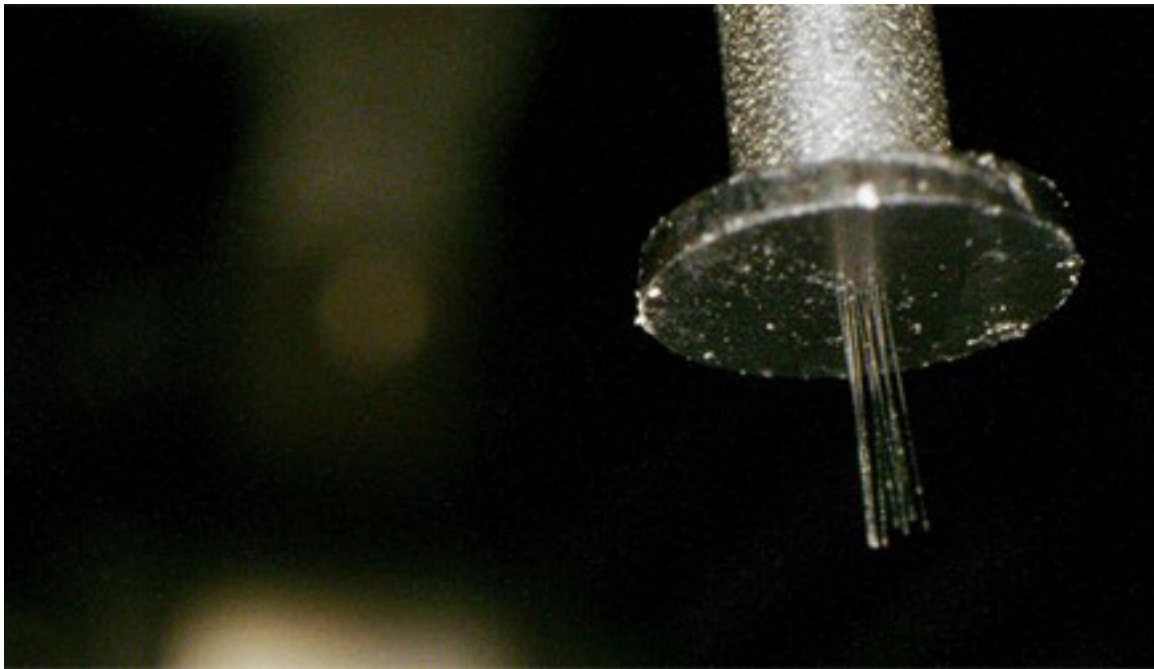
Thin carbon fibres act as active electrodes. Source: Lead entrepreneur Professor Steven Praver, University of Melbourne.
