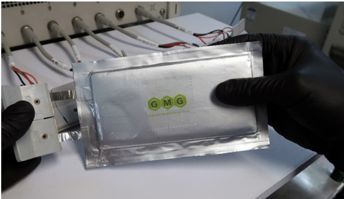
AIB 1Ah pouch cell. Source: Lead scientist Dr Xiaodan Huan, Graphene Manufacturing Group.
